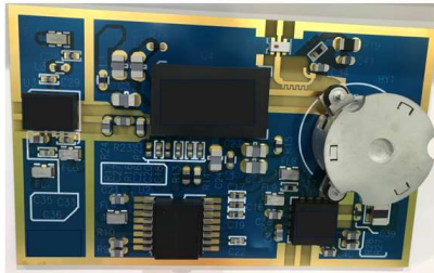
Example of 6GHz PA module with packaged GaN device size 80x40mm
